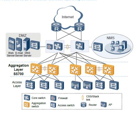
On an enterprise campus network, the S5720-SI series switches connect to access switches through GE or 10GE ports and connect to core switches through 10GE optical ports, providing high performance and large switching capacity. The network provides 10 Gbit/s rate for the backbone layer and 100 Mbit/s access rate for terminals, meeting requirements for high bandwidth and multi-service.
